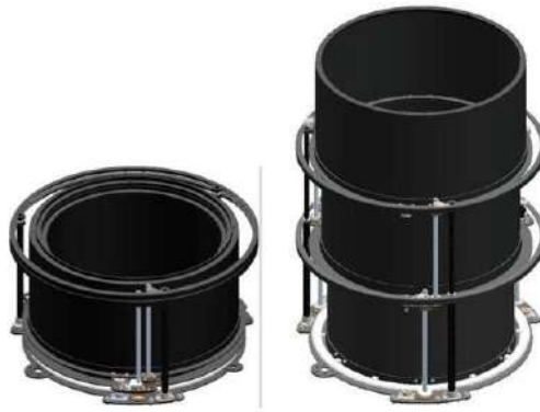
Figure 1.5. Deployable telescopic barrel, stowed (left) and deployed (right)
