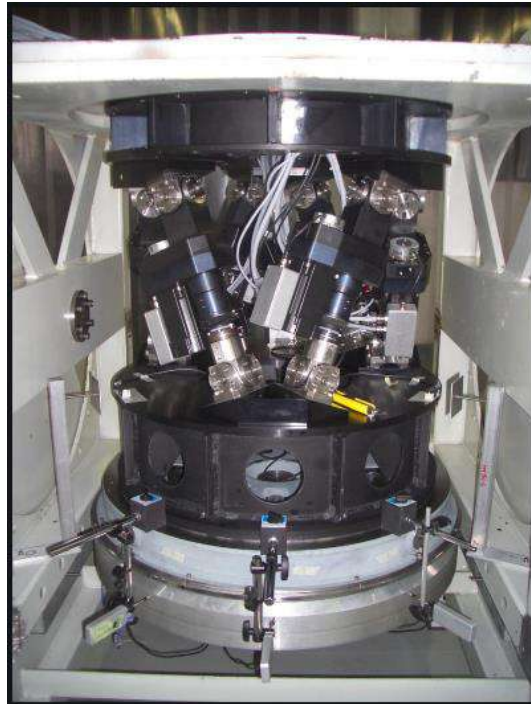
Figure 1.10. Active optics control of the secondary mirror
