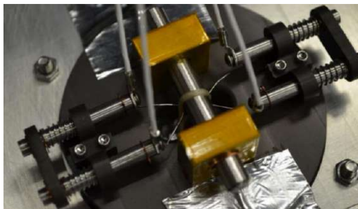
Figure 3.5. Assembled burn wire release mechanism
