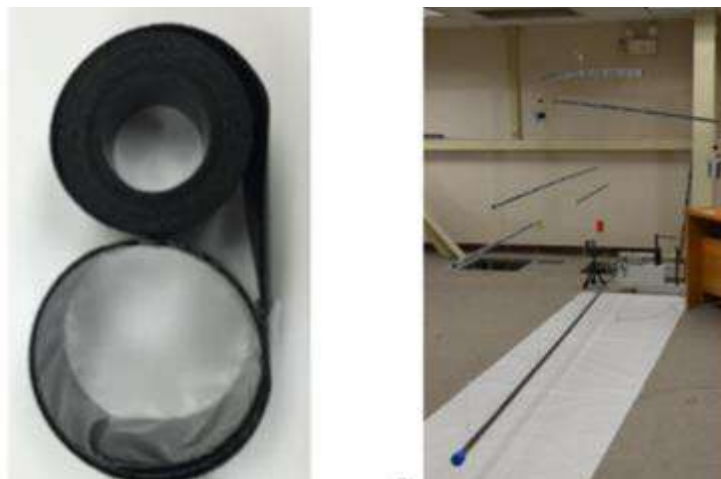
Figure 2.25. Shearless boom stowed, showing efficient coiling diameter (left) and deployed, with gravity off-loaded (right)
