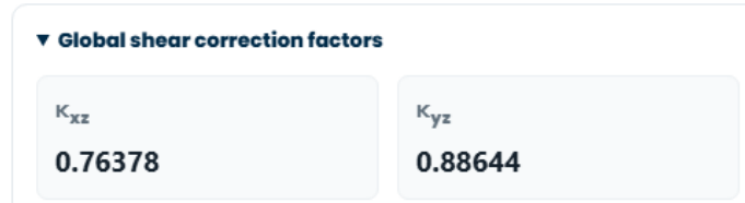
Figure 11: Expanded global shear-correction factor panel. The reported values are the global \kappa_{xz} and \kappa_{yz} factors used for the corrected FSDT calculation.
